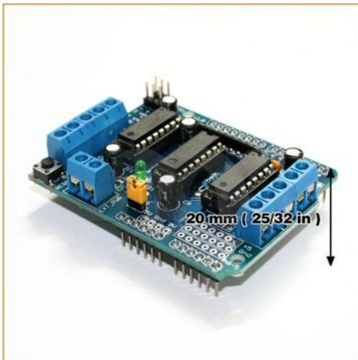
**L293D Motor Control Expansion Board Motor Drive Shield Packing include:**
